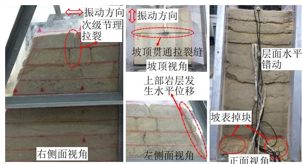
(a) 阶段1: 层间次级节理拉裂、岩层沿水平层面错动
